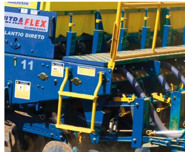
Drive Mechanism: Easy system, without use of tools, offers 43 different combinations for fertilizers and 23 for seeds distribution.
