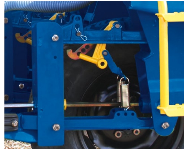
Drive Mechanism: Easy system, without use of tools, offers 43 different combinations for fertilizers and 23 for seeds distribution.
