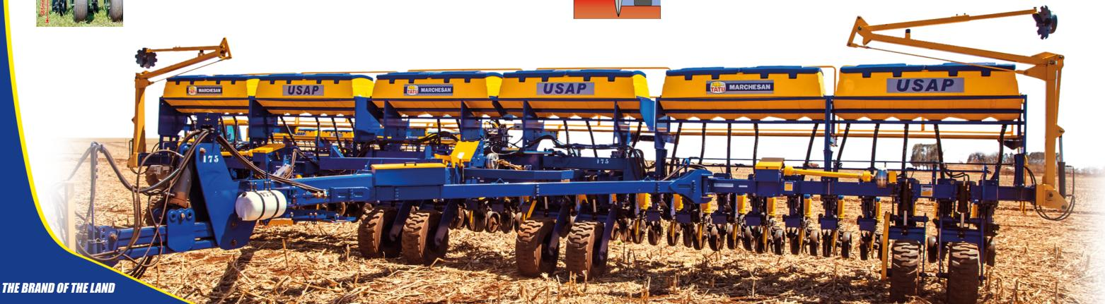
Concept for No-Till Planting: the distance between depth control wheel and the double discs assembly provides better conditions for planting in compacted soils, inhibiting the adherence of straw or clay soils to components of the planting line.
