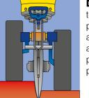
Depth control wheels: acting next to the seed double discs to control the proper depth of planting. Independent and vertical oscillations of the bands allow to follow the soli irregularities, providing an uniform emergence of the plants.
