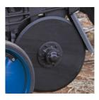
Unaligned double disc: make easy to open the furrow to get a homogeneous seed placement depth, providing an uniform seed germination.
