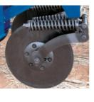
High cutting straw capacity: the assembly position of the double discs, allow a continuous operation and an excellent straw cutting even in soils with high level of residues. 18" Plain Coulter Blade: Allow lateral movements and adjustments on height to follow uneven ground in different situations and soil conditions.
