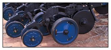
"V" Press Wheel Assembly: equipped with 5 adjustments levels. The press wheel make pressure in the superficial layer, eliminating air pockets, improving contact between soil and seed. The result is better seed distribution and germination.
