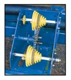
Transmission: equipped with exclusive TRA system, making possible a wide range of combinations for seeds distribution of different crops, without use of tools for changing to a desired sprockets.
