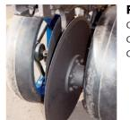
Reduced compaction: the assembly distance of control depth wheel and coulter blade assembly, prevent soil compaction.
