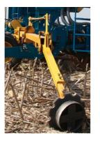
Row Markers: Tri-articulated, has hydraulic cylinders and adjustments for length and angle of the arm, forming a compact system for transporting.
